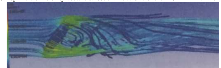
FIGURE 14 Top streamlined view of swirling vortex flow features and the velocity on the surface of 45° Open Butterfly Valve disc of MODEL-II
